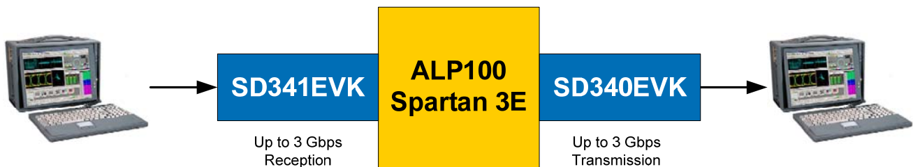
Figure 9) Pass-through Test Setup
